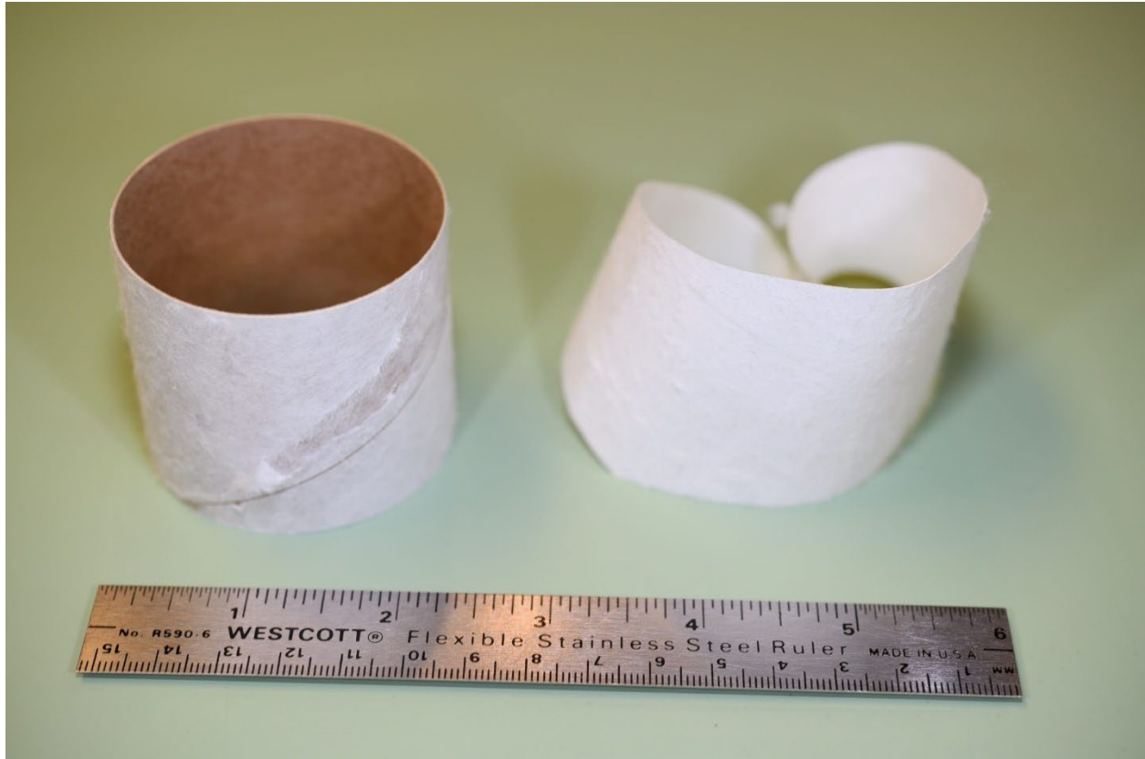
Photo 100: Instrumentation Section BT-70 Underlay
