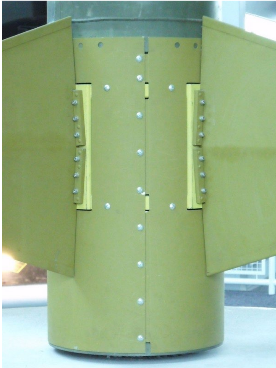
Photo 28: Booster Sleeve Seam
