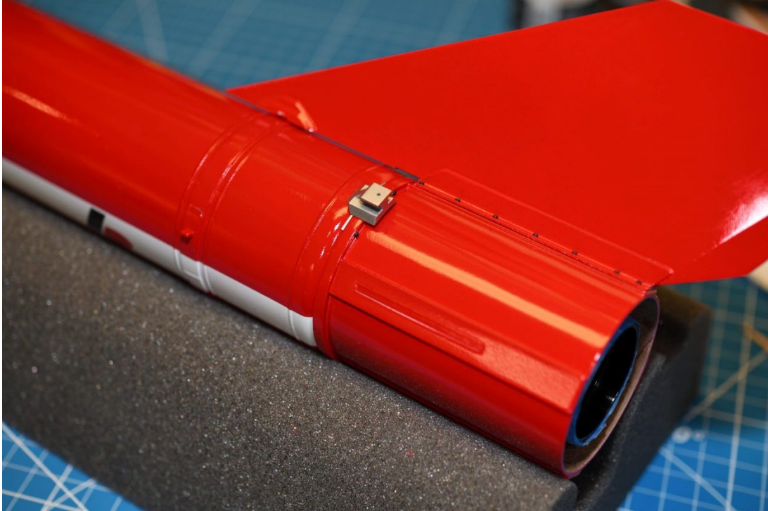
Photo 85: Finished Fin Installed
